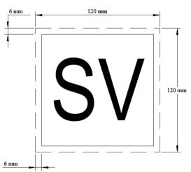
6.8.3.2.9.6.5 The material used shall be weather-resistant and it shall be ensured that the mark is durable. The mark shall not become detached from its mount in the event of 15 minutes' engulfment in fire. It shall remain affixed irrespective of the orientation of the tank.
